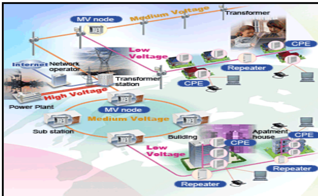
Figura 3. Esquema de red PLC Outdoor / Indoor. [CHIF2006]
